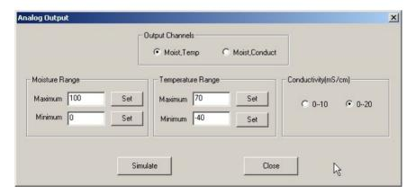
The conductivity range can be selected, depending on the specific soil which is measured. 0..20 dS/m should be selected for soils with a very high salinity content.
