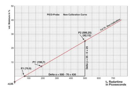
The coefficient m<sub>1</sub> is calculated from the slope of the curve Cal15:
