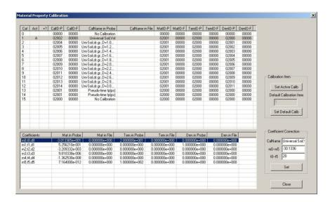
The desired and possibly altered calibration curve (Cal1. .15) which is activated after switching on the probes power supply can be adjusted with the button "Set Default Calib".
